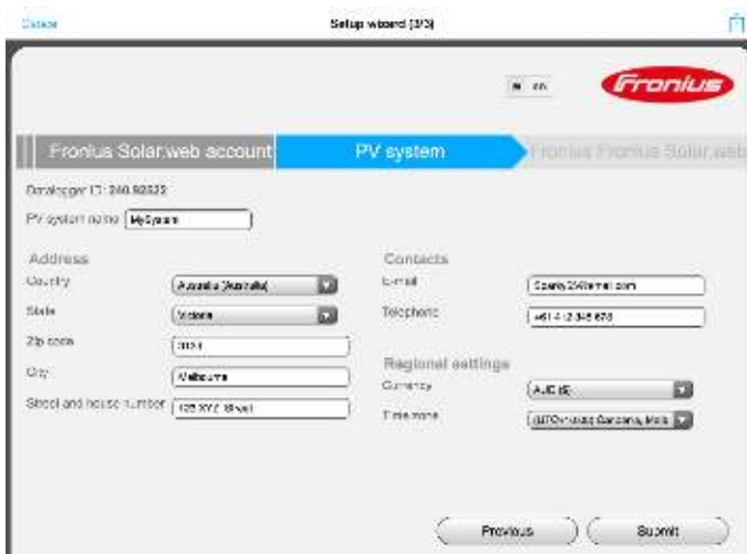
Fig.14: SolarWeb App – Adding a system to a SolarWeb account
