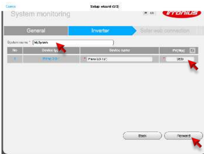
Fig.6: Fronius SolarWeb App Inverter Settings
