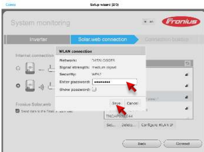
Fig.8: Fronius SolarWeb App Connection Settings - WiFi password
