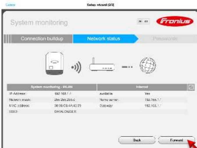
Fig.11: Wizard in Fronius SolarWeb App – Network status
